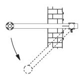
Rotates inboard to give safe access for camera servicing.
