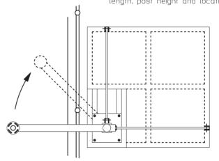
Rotates inboard to give safe access for camera servicing.
