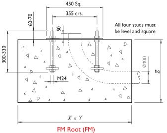
4-hole fixing - up to 8m 8-hole fixing - 10m
