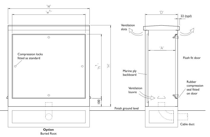
All our road side cabinets are constructed from stainless steel (3CR12) and powder coated with a black finish as standard
